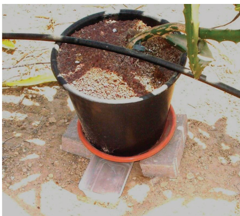
FIGURE 8 - Pitaya bucket in the orchard with a tray to collect and measure efflux of water and minerals.
